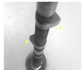
Fig. 4 Cam shaft of an E-Type Jaguar car engine. The arrowheads show two of the cam lobes.
